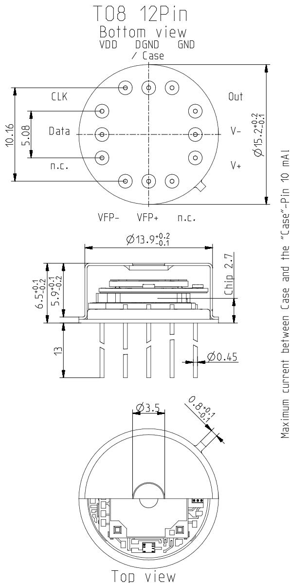
Maximum current between Case and the "Case"-Pin 10 mA!
