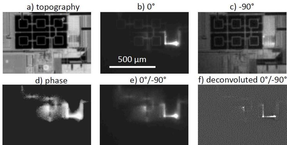
**Fig. 8.** (a) Topography image, (b)  $0^\circ$  image, (c)  $-90^\circ$  image, (d) phase image, (e)  $0^\circ/-90^\circ$  image, and (f) spatially deconvoluted  $0^\circ/-90^\circ$  image of a region in a bare IC.
