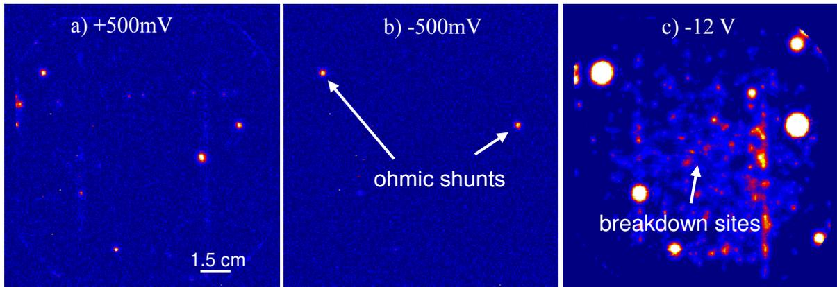
**Fig. 4.** (a) Forward bias and (b) low reverse bias LIT amplitude image showing shunts with linear and non-linear characteristic, (c) high reverse bias amplitude image showing in addition breakdown sites.
