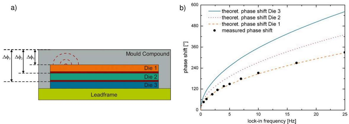
**Fig. 9.** (a) Cross section through a stacked IC, (b) simulated (theoretical) phase shift for a defect lying in different dies of the IC and measured phase shift values for different lock-in frequencies.
