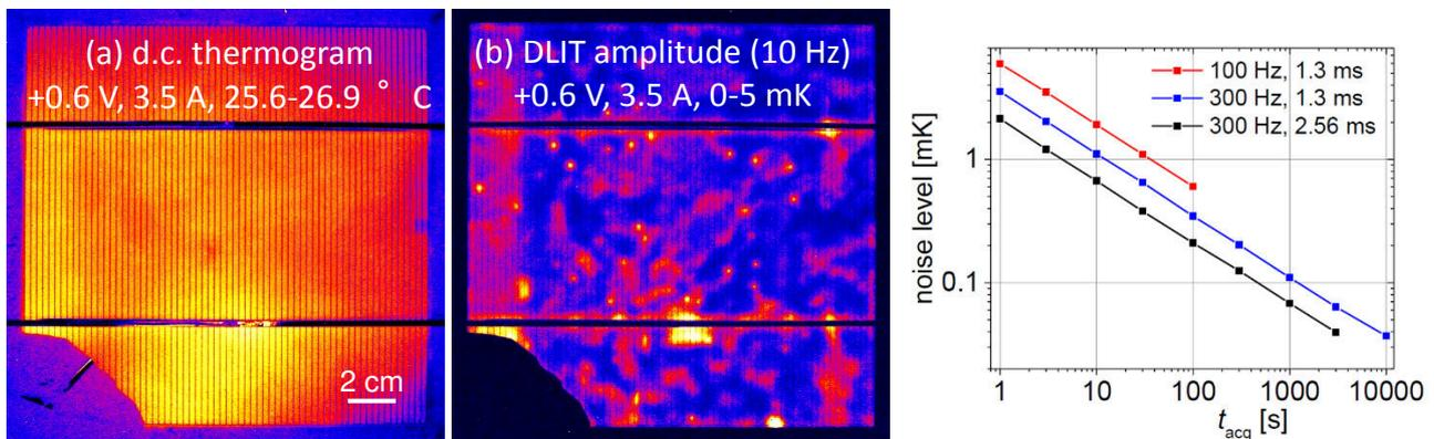
**Fig. 3.** (a) Steady-state (d.c.) thermogram and (b) dark lock-in thermography image of a solar cell under identical conditions, (c) measured amplitude noise levels of the InfraTec PV-LIT system.
