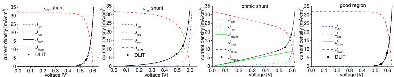
**Fig. 6.** Thermally measured dark and illuminated local I-V characteristics of different positions in a solar cell ( $J_{diff}$  shunt,  $J_{rec}$  shunt, ohmic shunt, and a good region).
